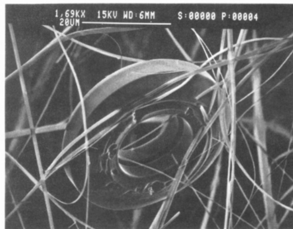
Figure 4. In contrast to Figure 3, this SEM view shows a "smooth" \text{NbSe}_3 object which is remarkably featureless, i.e., no bands, but it does have a curious inner void.
